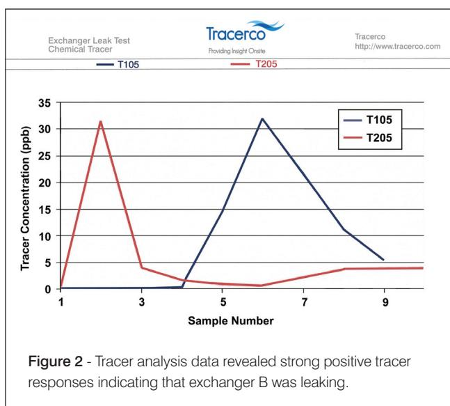
**Figure 2** - Tracer analysis data revealed strong positive tracer responses indicating that exchanger B was leaking.
